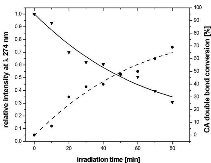
**Fig. 4.1.** The dependence of the relative intensity of the absorbance cinnamate groups in the copolymer and conversion of cinnamate groups depending on the UV exposure time
