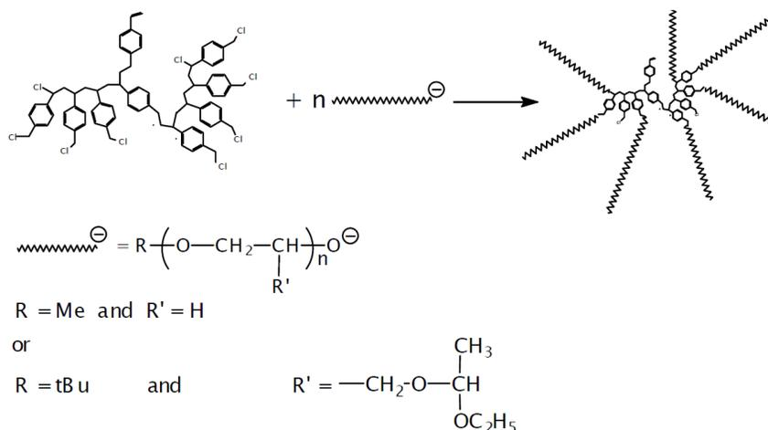
**Scheme 3.1.** Termination of the living polyoxirane chains with branched poly(*p*-chloromethylstyrene) core
