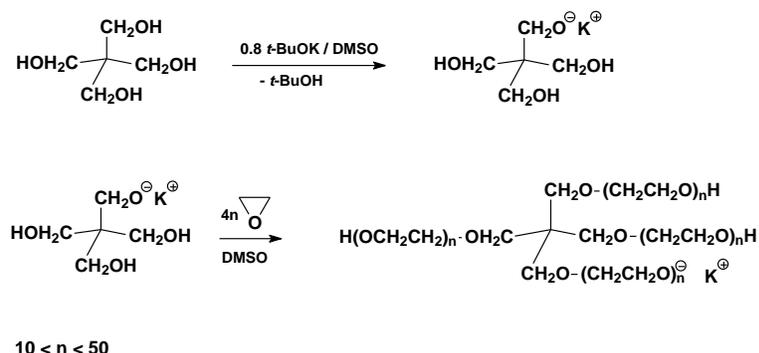
**Scheme 2.5.** The synthesis of star polymers of ethylene oxide
