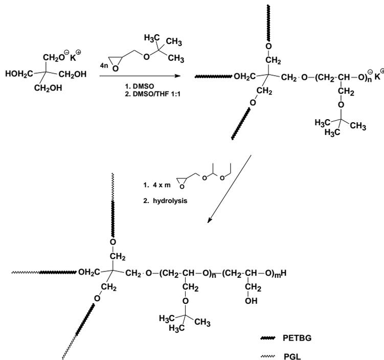
**Scheme 2.8.** Synthesis of star copolymers of poly(*tert*-butyl glycidyl ether) – block – polyglycidol arms
