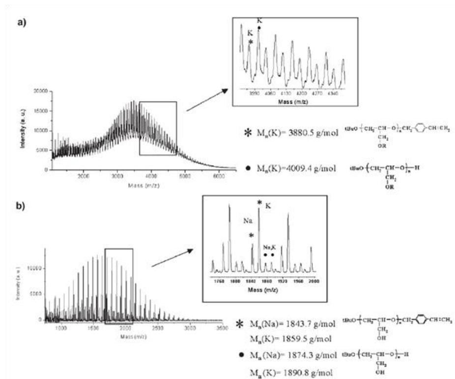
**Fig. 3.2.** MALDI-TOF spectrum: a) macromonomer PEEGE-St and b) macromonomer PGL-St – after deprotection of the EEGE block
