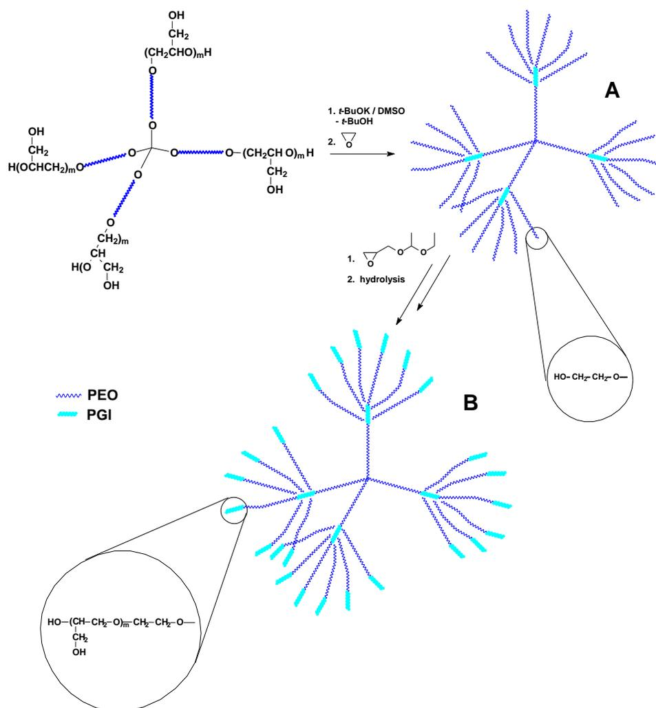
**Scheme 2.7.** Synthesis of the dendritic star copolymers of ethylene oxide and glycidol
