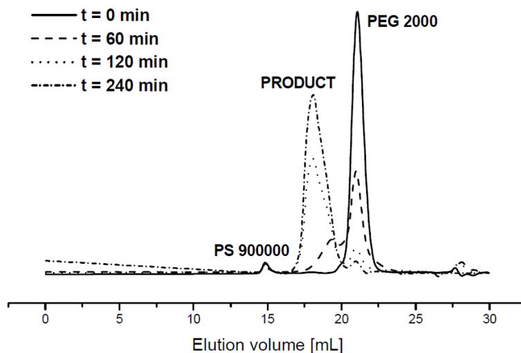
**Fig. 3.1.** SEC chromatograms of the reaction mixture PEO 2000 g/mol with a branched core of poly(*p*-chloromethylstyrene) for various reaction times
