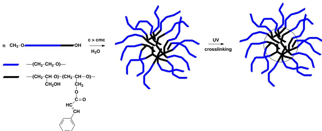
**Scheme 4.3.** Formation and stabilization of amphiphilic PEO-b-(GI-co-CGI) copolymer micelles with cinnamate groups
