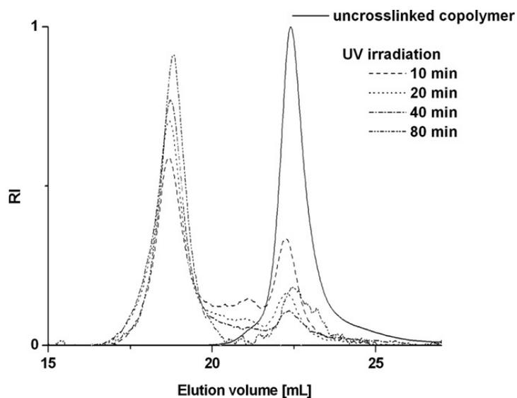
**Fig. 4.2.** SEC chromatograms of the copolymer after various exposure times of the micelles formed in water. Non-crosslinked micelles disintegrate under SEC analysis conditions and appear as a signal derived from the copolymer
