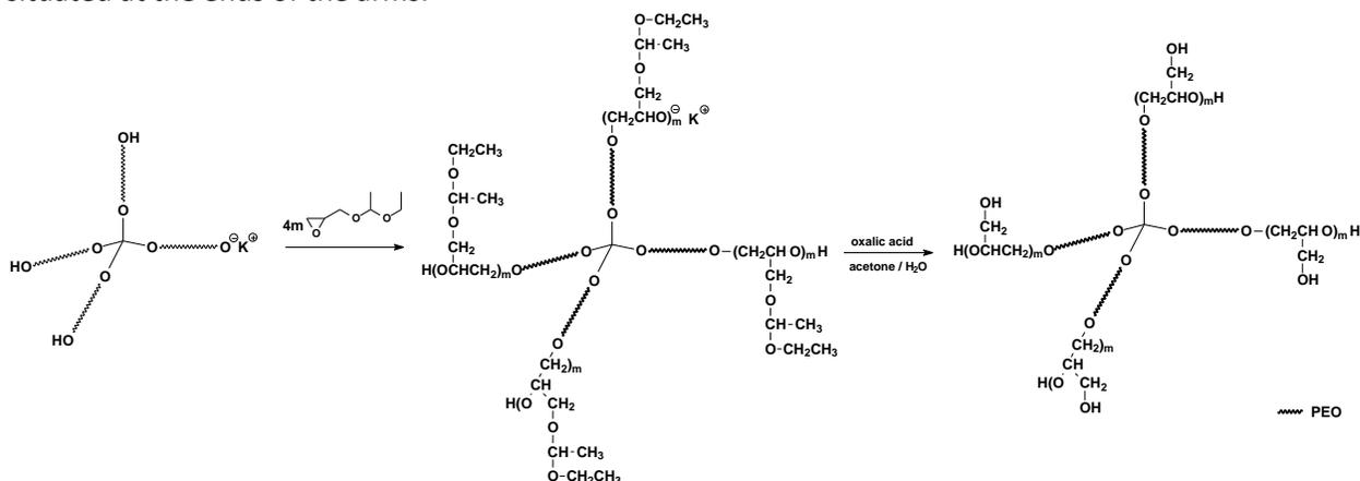
**Scheme 2.6.** The synthesis of star block copolymers of ethylene oxide and glycidol
