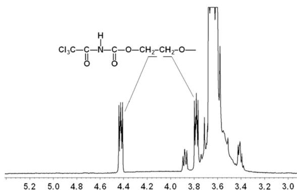
**Fig. 2.4.** <sup>1</sup>H NMR (CDCl<sub>3</sub>, 300 MHz) spectrum of the dendritic star copolymer A/30 (see Table 2.6) after reaction with the trichloroacetylisocyanate
