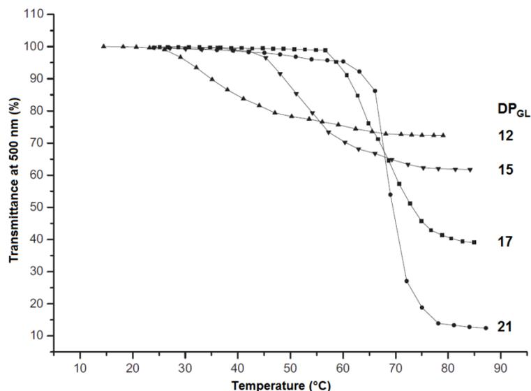
**Fig. 2.6.** Dependence of transmittance on the temperature of the water solution of star copolymers of poly(*tert*-butyl glycidyl ether) – block – polyglycidol arms of DP of glycidol block: 12, 15, 17 and 21
