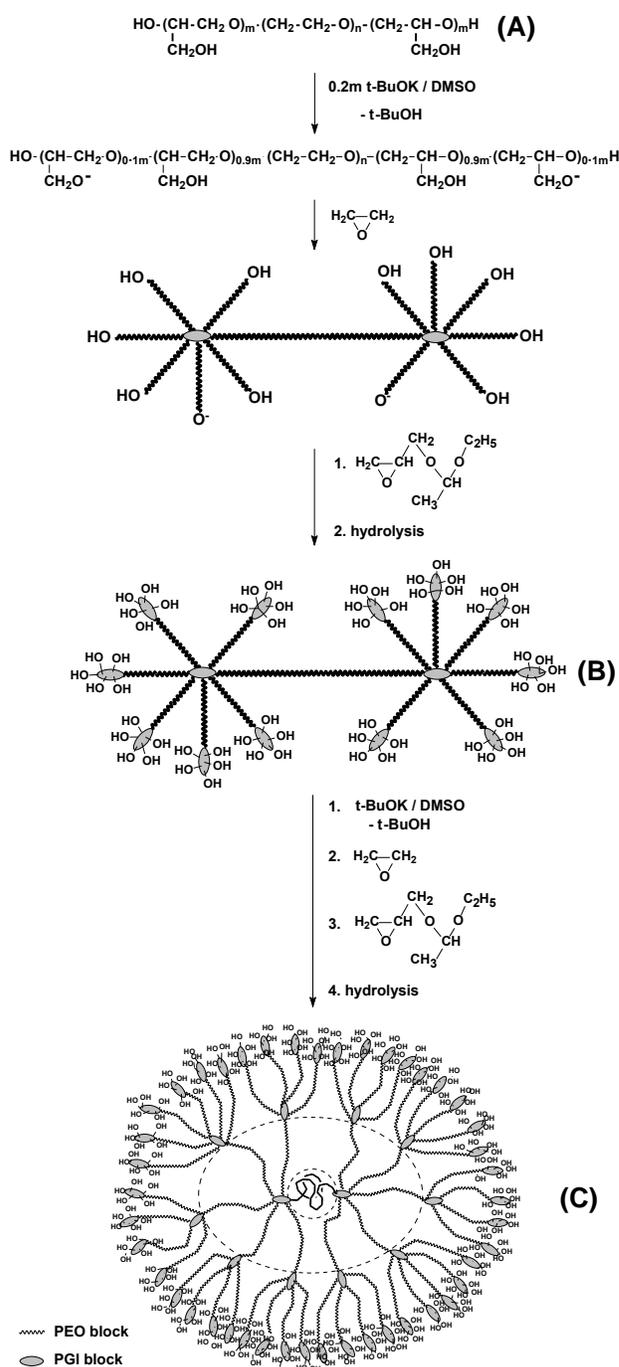
**Scheme 2.4.** Stages of the synthesis of branched copolymer of ethylene oxide and glycidol of “pom-pom” chain structure
