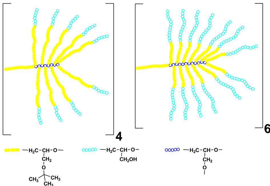
**Fig. 2.9.** Comparison of the arm structures of dendritic block copolymers of *tert*-butyl glycidyl ether and glycidol from position 1 and 4 of table 2.9
