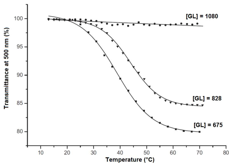
**Fig. 2.9.** The dependence of transmittance on the temperature of aqueous solutions of dendritic copolymers of *tert*-butyl glycidyl ether and glycidol. The value of [GL] corresponds to the number of glycidol units in the outer shell of the copolymer
