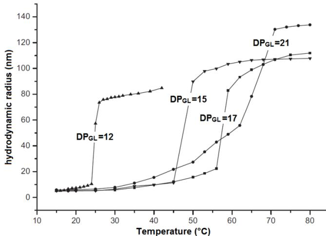
**Fig. 2.7.** The dependence of the hydrodynamic radius of star copolymers of arms of poly (*tert*-butyl glycidyl ether) – block – polyglycidol, with the DP of polyglycidol block:12, 15, 17 and 21 units in the water solution, on the temperature (concentration 2 g/L)
