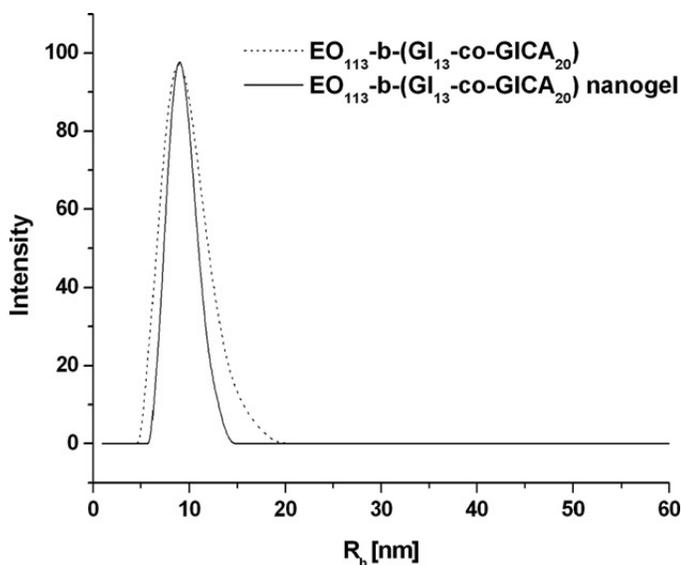
**Fig. 4.3.** Hydrodynamic radii  $R_h$  (25 °C, water) of copolymer Me-EO<sub>113</sub>-b (GI<sub>13</sub>-co-CGI<sub>20</sub>) before and after stabilization of the micelle
